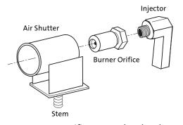
Figure 12. Burner orifice removal and replacement.
